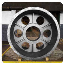
Pulley, 2,000 kg Drive for mills, granulator machines and crushers
